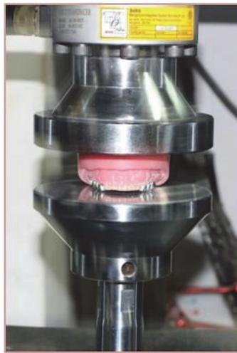
Fig.4 Cyclic loading using a universal testing machine
