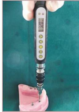
Fig.2 Digital torque driver
