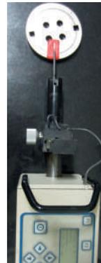
Fig. 8: Roughness of prepared specimens measured using contact profilometer
